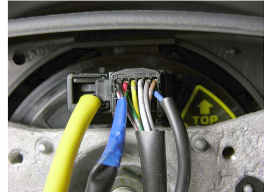
Connector behind the airbag (Viewed from wire side)
