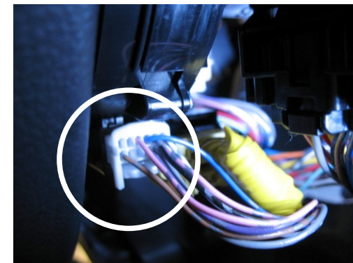
Mount the White/Purple and the Black wire with terminals crimped on into the connector on the clock spring in pin 4 and pin 5. Placement is unimportant
