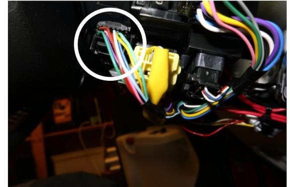
Plug in White wire in pin 5, and solder together with White / purple wire.
