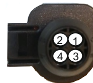
Brake light switch. on the side of brake master cylinder. (Viewed from wire side)
