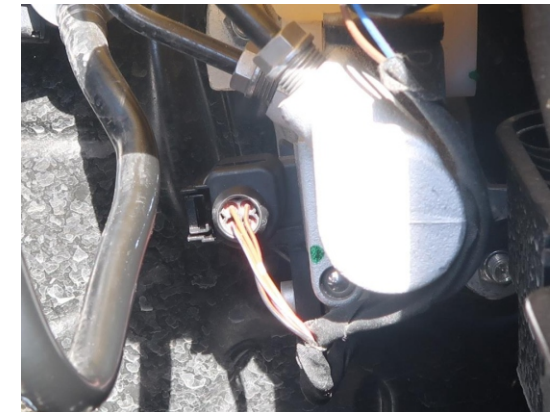
Brake light switch on the side of the brake master cylinder in the engine bay.
